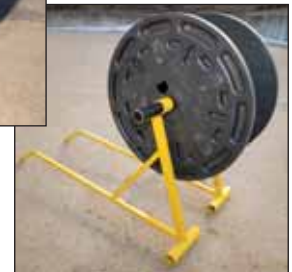
3) Cable can now be pulled off in the direction of the handles
