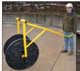
1) After sliding the frames onto the spindle bar, maneuver the reel into position
