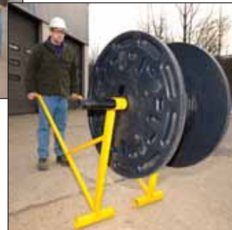
2) Rotate the handles around the spindle and lift the drum into position
