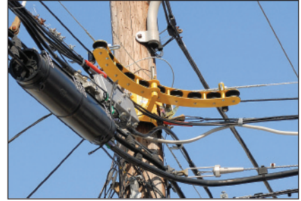
Photo Caption: The 45° Corner Cable Block from General Machine Products Company in action.
