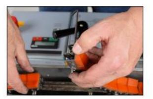
11. Pass the pre-lubricated new chain around the drive sprocket. Feed the chain along the unit and reconnect the chainconnecting link. Remember to install the 2 center connecting link plates. 10. Check the chain support slide bars for wear. Clean and relubricate.
