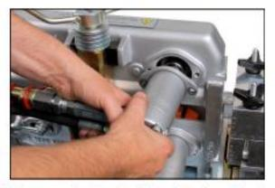
1. Remove the hydraulic motor from the top frame using 6mm Hex Key. Do not disconnect hydraulic hoses connected to the motor. key.
