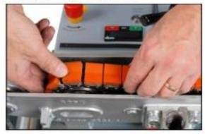
12. Align the tension sprocket with the chain and locate into position. Insert the tension pin through the tension sprocket. Place the tension pin spacer on the tension pin through the opposite hole. Refit swing bolts using a 13mm wrench. Adjust the chain evenly via the swing bolts, checking free rotation of the chain. Do not over tighten the chain.
