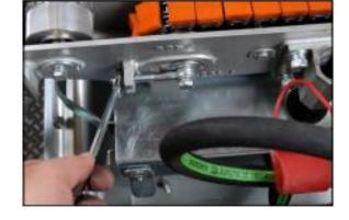
3. Unscrew the main clamping screw and separate the top and the bottom of the pusher unit. Place in a safe location.
