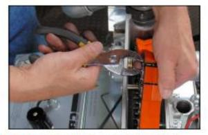
8. Remove the chain-connecting link.
