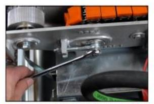
Remove the swing bolt from the side of unit using a 13mm wrench.
