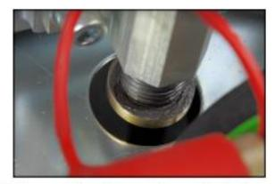
Remove the stop washer on the bottom of the main jacking screw using a 6 mm Hex key.
