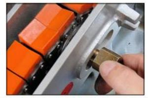
Pull the tensioner pin out from the sprocket assembly. Remove spacer from other side.
