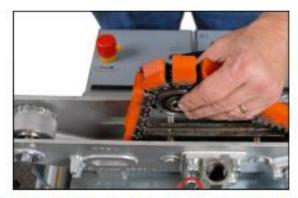
7. Remove the tension sprocket assembly
