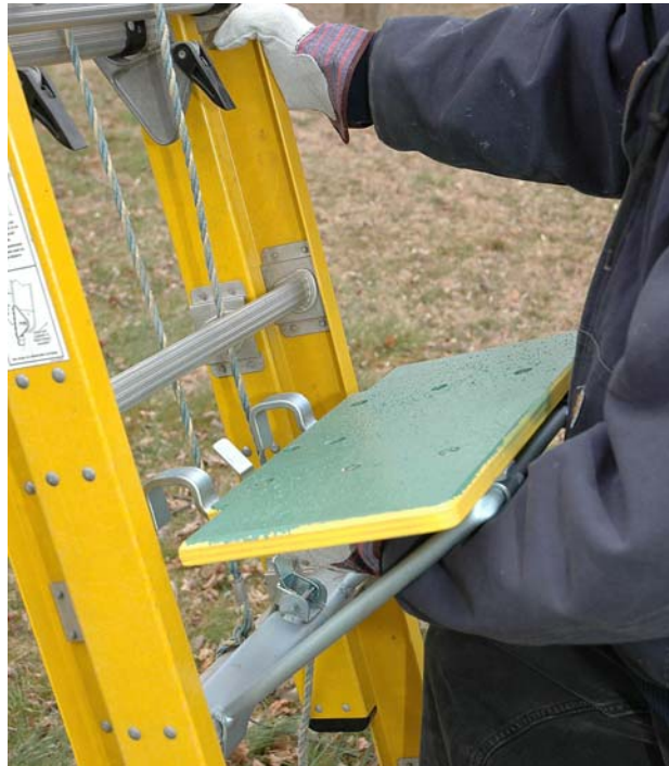
The frame is equipped with hooks and spring-actuated latches which lock the frame to the rungs of the ladder.
