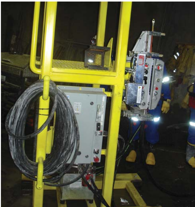
Vertical Rod Pusher and electric hydraulic power pack mounted on Cameco-fabricated deployment frame.
