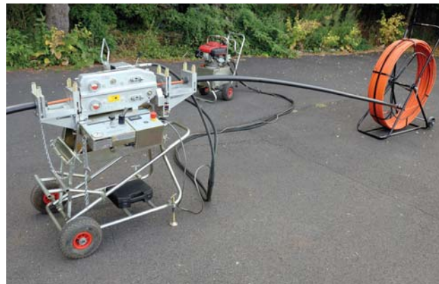
The Portable Powered Duct Rod Pusher by General Machine Products Co.
