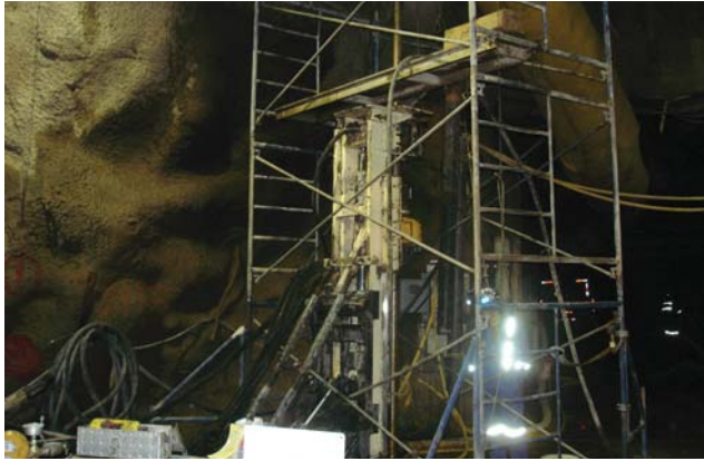
The GMP Vertical Rod Pusher frees up geotechnical drills, such as the one shown here, from survey tool deployment assignments.
