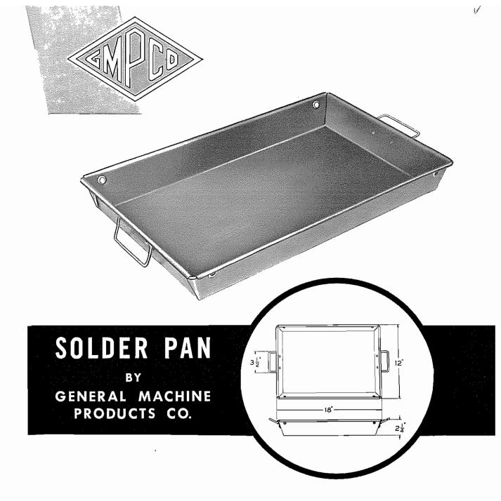
This lightweight sheet-steel pan is made for catching solder drippings when wiping joints in cable splicing operations. The pan has folded corners, a folding loop handle at each end and is provided with eyelets near each corner for safely suspending the pan under the cable.
