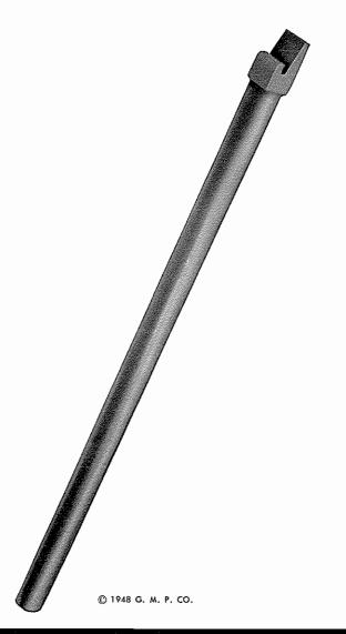
The pipe spreader quickly and easily enlarges the slot produced by the pipe ripper in order to facilitate the removal of conduit from a cable. The hardened steel fork engages the edges of the pipe wall at the slot. The handle is made of 1 ½" steel pipe for lightness and also so that a bar may be inserted when greater leverage is required.
