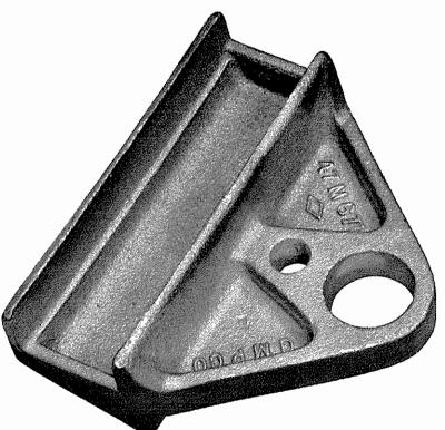
This is a malleable iron casting with a pocket for holding guy clamps while tightening the bolts when assembling the clamps with strand. It is provided with a 1 5/16-inch hole for attachment to the rear end of the truck with the truck eyebolt. Lugs which bear against the edge of the scuffle plate prevent rotation of the holder. A 9/16-inch hole is also provided to permit attachment of the holder to the truck vise bracket with a 1/2-inch machine bolt.
