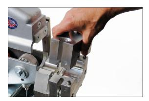
15. Select the correct size cable infeed collet to suit the size of the cable to be installed and secure with the cap screw into each housing. Note: Sealing cord is not required on this collet.
