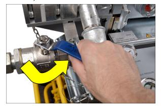
5. Turn the speed control valve towards "MAX" until the required speed is achieved
