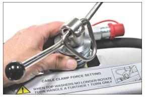
Tighten the handle with one hand while rotating the clamp washers with the other. The clamp washers will turn easily until the handle begins to clamp them. When the clamp washers become almost impossible to turn with one hand this is the start point for the clamp force setting. Continue to turn the handle a further 1 full turn. This will ensure the correct cable clamp force.
