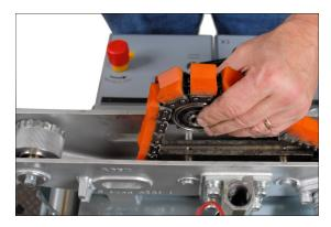
7. Remove the tension sprocket assembly
