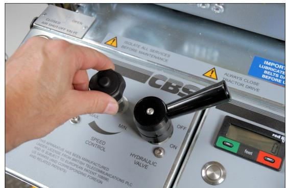
39. Turn the air valve to the “closed” position. Allow the air pressure to exhaust. This may take several minutes as there may be a considerable amount of air in the sub-duct. Do not open the air chamber until the air pressure gauge reads **Zero**.
