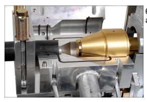
6. Fit the upper cable guide collet ensure both seals are correctly located.
