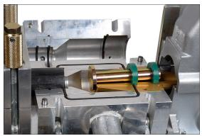
5. Fit the cable seal plug and two cable seals (coated with silicon grease) into the lower half cable seal collet. Ensure that the split of the innermost seal is in the lower half of the air chamber slightly rotated from the vertical. The split of the outer most seal is also in the lower half of the air chamber slightly rotated from the vertical in the other direction to the innermost seal. Both grooves face away from the tractor drive.
