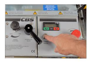
The display will indicate the speed and distance travelled by the cable. To toggle between speed and distance press the SEL (green) button. R displayed on the left side of the screen designates speed (rate). To reset the distance press RST (red) button.
