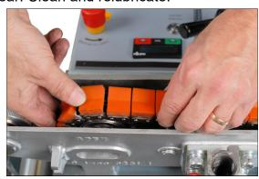
12. Align the tension sprocket with the chain and locate into position. Insert the tension pin through the tension sprocket. Place the tension pin spacer on the tension pin through the opposite hole. Refit swing bolts using a 13mm wrench. Adjust the chain evenly via the swing bolts, checking free rotation of the chain. Do not over tighten the chain.
