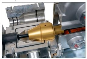
22. Fit the upper cable guide collet in po- 23. Re-fit the air chamber lid ensuring correct location on the dowels and tighten down the 4 retaining knobs.
