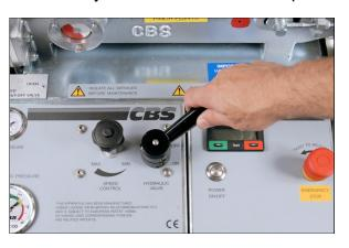
Turn the speed control knob to "MIN" position (fully counter clockwise)
