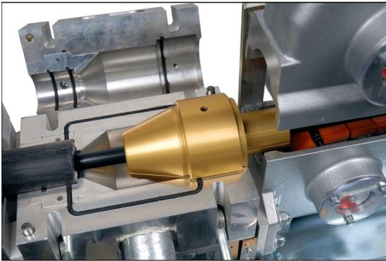
23. Re-fit the air chamber lid ensuring correct location on the dowels and tighten down the 4 retaining knobs.
