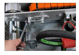
4. On the lower unit, slacken the 2 chain adjusters using a 13mm wrench.
