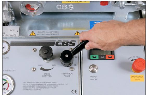
38. Turn the speed control knob to the “MIN” (counter clockwise) and press the reset button.
