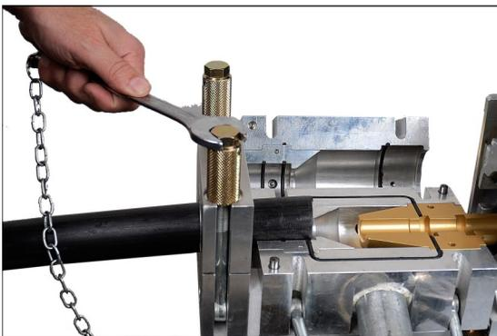
4. Clamp the sub-duct and tighten the two retaining nuts just enough to secure the duct. (Over tightening could strip the threads on the clamps)
