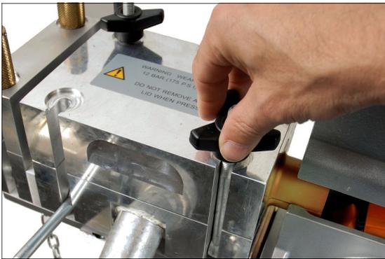
7. Re-fit the air chamber lid ensuring correct location on the dowels and tighten down the 4 retaining knobs.
