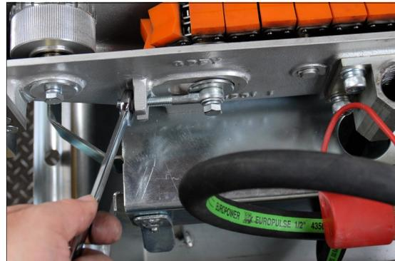
3. Unscrew the main clamping screw and separate the top and the bottom of the pusher unit. Place in a safe location.
