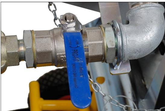
17. When the foam plug has been expelled from the end or the sub-duct, turn the air valve to the “closed” position and shut down the compressor. **Allow the air chamber and sub-duct to exhaust all the compressed air. Note: Never open the air chamber until the air pressure gauge reads zero.**
