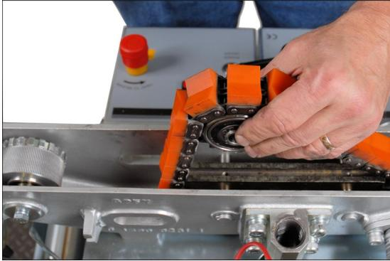
7. Remove the tension sprocket assembly
