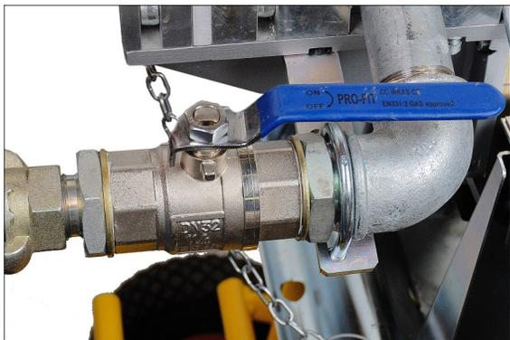
11. Confirm that air is being expelled from the far end of the sub-duct under pressure. If not this indicates the run is too long, there is leak, an obstruction or the sub-duct is crushed or otherwise damaged or disconnected. This must be remedied before any cable blowing is undertaken, when confirmation is received, turn the air valve to the “closed” position and shut down the compressor.
