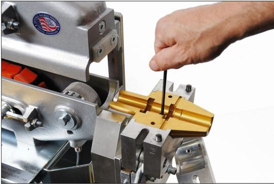
**Always check and verify the correct size collets are fitted before operating the blowing machine.**
