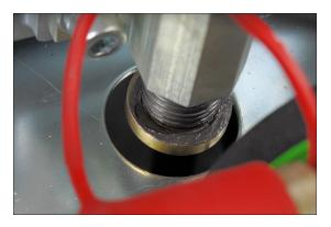
2. Remove the stop washer on the bottom of the main jacking screw using a 6 mm Hex key.
