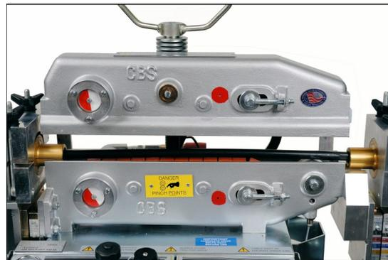
Close the infeed cable guide upper housing and secure with the swing bolt and thumb nut, ensure the cable is correctly located in the bore of the collet.
