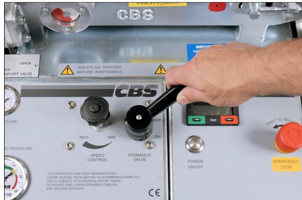
Turn the speed control knob to "MIN" position (fully counter clockwise)
