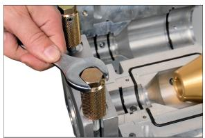
For cables 6 - 12mm O.D. these settings need to be changed, refer to the section 4 "SPECIFICATION" for the correct pressure settings for the relief valve and pressure switch and to section 6 "MAINTENANCE" for the pressure setting procedures.
