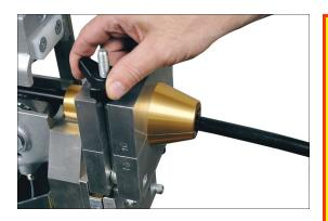
Note: Ensure that the compressor air supply is never allowed to enter the air chamber or subduct when the top tractor drive frame is in the upper position. (i.e. not clamping the cable) and / or the infeed guide bracket is open or not correctly secured.
