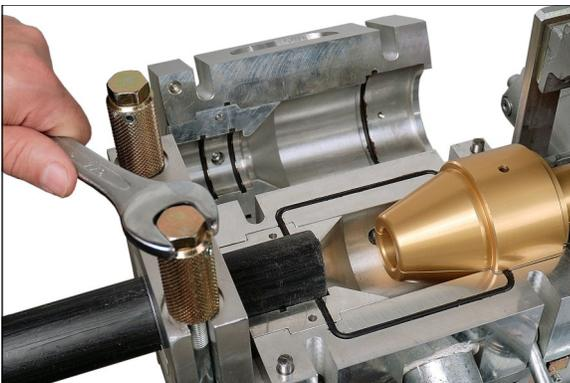
11. Clamp the sub-duct and tighten the two retaining nuts. Remove the upper cable collet.
