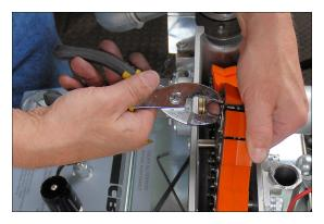
8. Remove the chain-connecting link.
