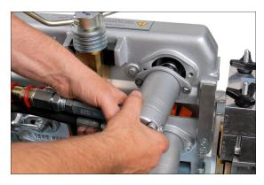
1. Remove the hydraulic motor from the top frame using 6mm Hex Key. Do not disconnect hydraulic hoses connected to the motor. key.
