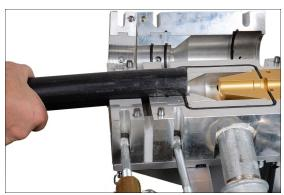
3. Open the sub-duct clamp and place the sub-duct into the sub-duct seal collet and sub-duct clamp collet. Ensure the sub-duct is fully engaged into the sub-duct seal collet.
