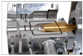
2. Clean the air chamber with a dry cloth, fit the correct size cable seal collet, sub-duct seal collets and sub-duct clamp collets refer to sections 8 & 9 and appendices 7 & 8 for further details. The collet with the horizontal "O" Ring grooves is fitted into the base of the air chamber and secured with a cap screw. Refit the radial seal cords
