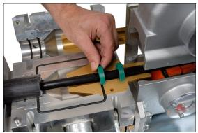
21. Install the second seal into the outer groove with the seal split in the lower half of the air chamber rotated slightly to the other side of the vertical (compared to the first cable seal). Ensure the groove seal lip is away from the tractor drive facing the sub-duct.
