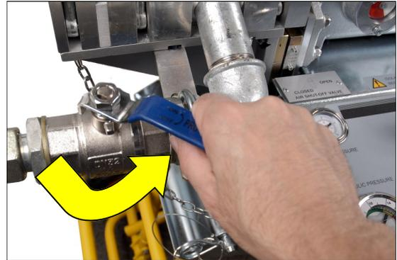
37. When the cable has reached its destination, the worker stationed at the other end of the duct will notify the operator to stop the machine by turning the hydraulic valve to the off position.
