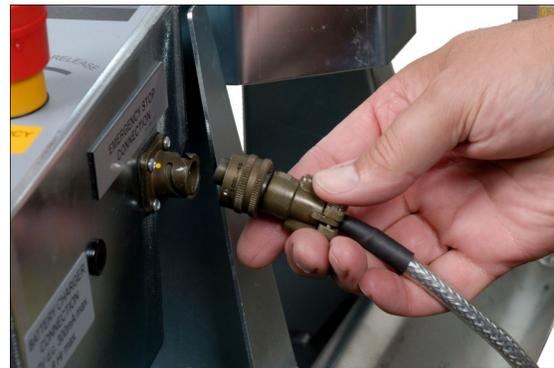
27. Connect the two hydraulic hoses and the emergency stop cable from the power pack (or hydraulic power source). Never run the blowing machine without the emergency stop cable being connected. **NOTE: Only authorized, fully trained operators should be allowed to operate the hydraulic power pack (or hydraulic power source).**
