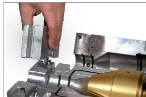
10. Place the sub-duct into the sub-duct seal collet and sub-duct clamp collet. Ensure the sub-duct is fully engaged into the sub-duct seal collet.
