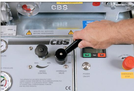
25. The speed control knob is in the "MIN" position (fully rotated counter-clockwise).
