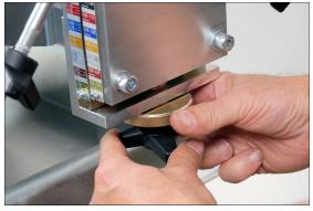
a 12-16mm cable collet range with a 16mm O.D. cable or blue to blue for a 16-20mm cable collet range with a 16mm O.D. cable. When the correct setting is achieved hold the adjusting screw and turn the locking clock wise to lock in position and prevent any movement during installation. (Refer to section 11 for details).
