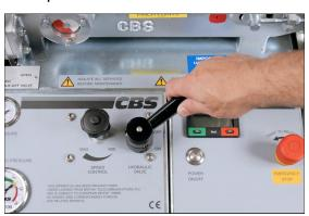
25. The speed control knob is in the "MIN" position (fully rotated counter-clockwise).
