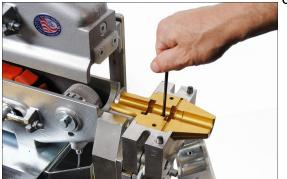
Always check and verify the correct size collets are fitted before operating the blowing machine.
