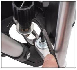
Securely attach Post and Bracket assembly to tripod with screw and washer provided using a 6mm hex wrench.
