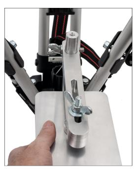
Slide tray and bracket assembly over post and tighten wing nut as shown in photo
