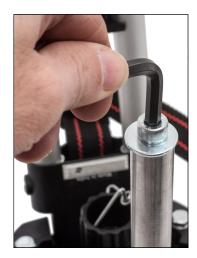
Remove screw and washer from end of post and bracket assembly using a 6mm hex wrench
