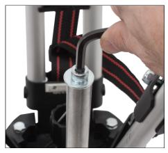
Replace screw and washer on end of post and bracket assembly using 6mm hex wrench
