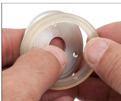
Remove the old silicone tire
