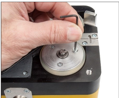
Remove all six M3 countersunk screws.
