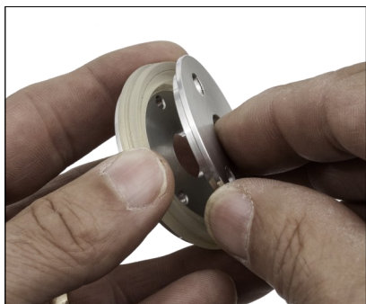
Separate the top and bottom support wheels.
