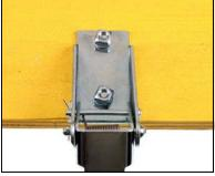
**STEP 4** Turn seat over and place back on wood blocks. Install bracket and latch assembly. Fasten with lock washers, nuts and tighten to 50 inch pounds.
