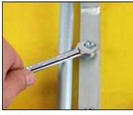
**STEP 5** Install frame assembly and fasten with lock washers, nuts and tighten to 50 inch pounds.
