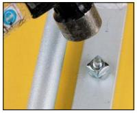
**STEP 6** Round over threads with a ball peen hammer on all bolts to prevent the nuts from backing off during use.
