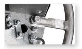
Insert the bolts through their mounting holes and tighten firmly using a wrench. Do not over tighten.
