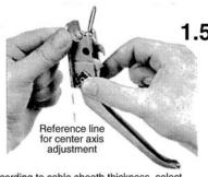
According to cable sheath thickness, select position I, II, III, or IIII by turning the center axis with thumb and forefinger.
