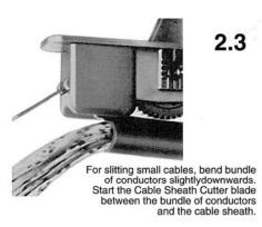
Support the cable and apply pressure to the body of the cutter with one hand. Next, push the handle of the tool down to pull the blade through the cable sheath. The serrated edges of the handle will pull the tool along the cable sheath.
