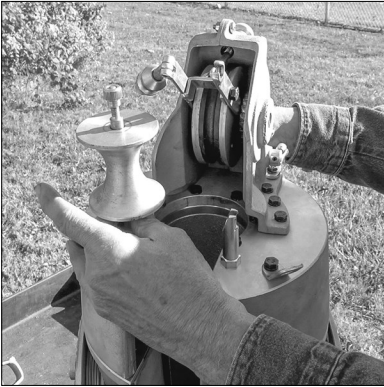
10. Open front lifter roller and retract and open the pressure roller. The lifter roller is detented and will stay open while you insert your cable.
