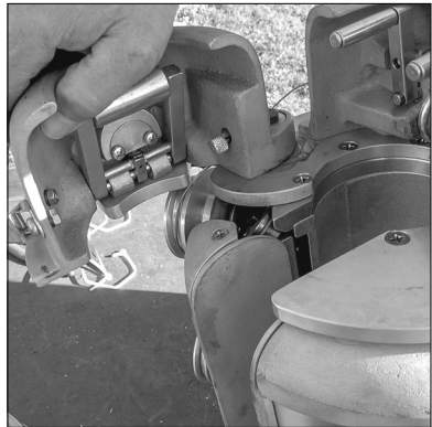
11. Open the rear gate. To close, use the release button shown with arrow. Open the guide rollers as far as they will go.
