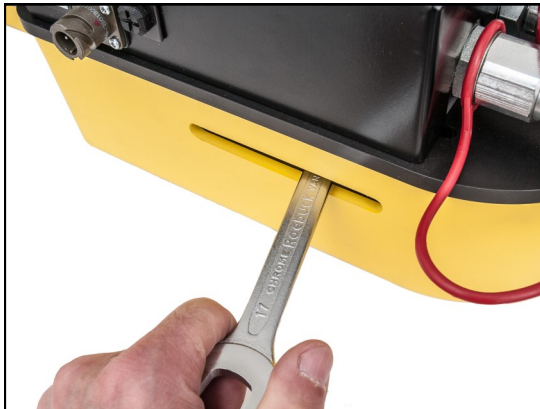
Loosen lock nut on pressure relief valve
