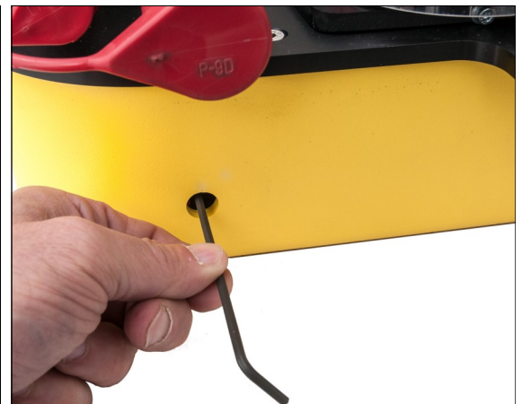
Pressure switch adjustment access hole found on side of unit
