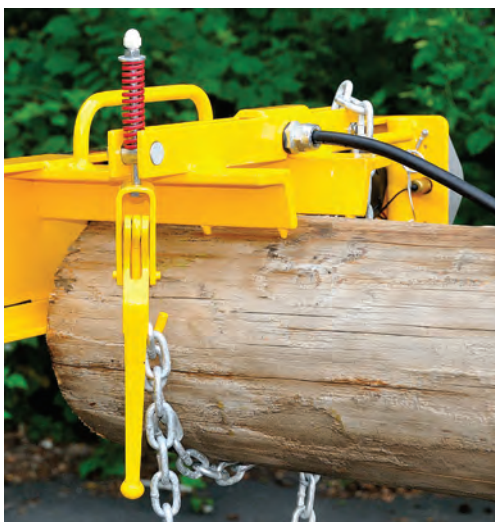
Chain Binder mount for wooden poles only.
